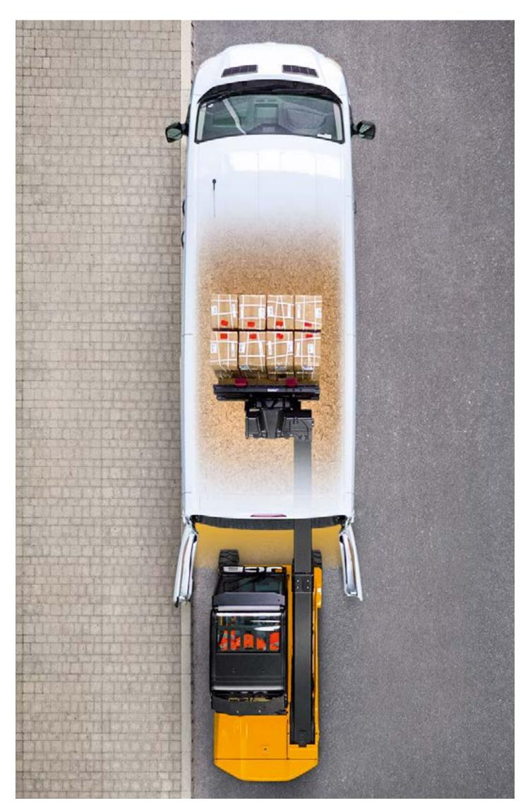
The unique telescopic boom saves 70m<sup>2</sup> of space per truck with single side loading. A low 2.2m cab height allows loading and unloading inside containers and trailers.
