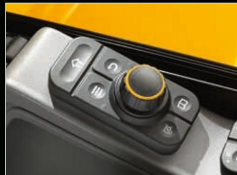
Tactile rotary controller provides precise intuitive control for the all new 7" colour display.
